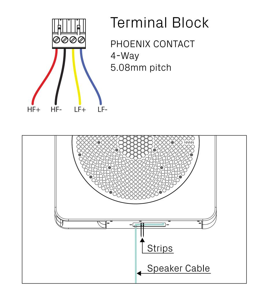
Thread the cable through the cable slot in the back cover of the Comium 30. Secure the cable with the Zip Ties. When the cable is in place, attach the Euro Block connector to the cable as in the figure above.
